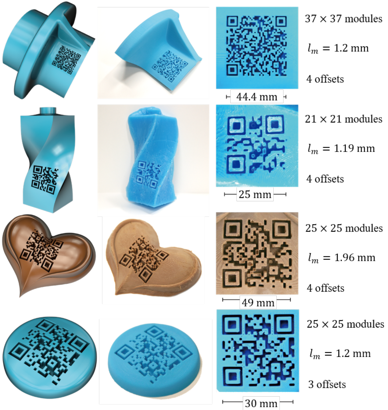
Figure 12: Top-to-bottom: FLANGE, PERFUME bottle, heart-shaped CHOCOLATE models, and Pharmaceutical TABLET. Left-to-right: Rendering, 3D printed model, closeup view of 3D QR code of 3D printed model.
