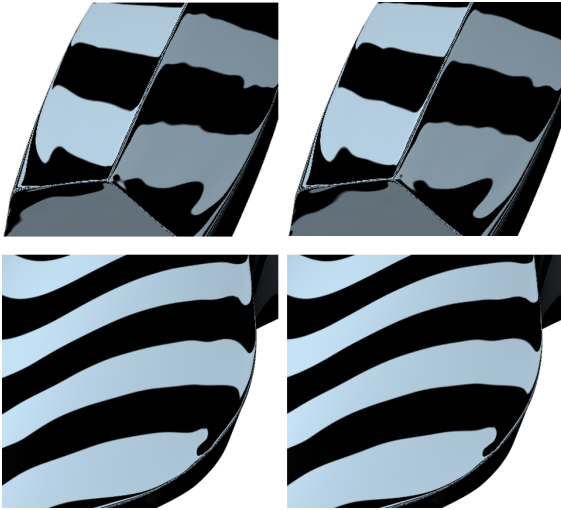
Figure 7: Visual comparison of BOAT (top) and MOUSE (bottom) surfaces fitted with adaptive tessellation (left) and uniform tessellation (right).
