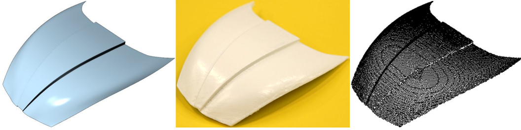
Figure 3: Automobile HOOD model. Left-to-right: Ground truth B-spline surface model, created by a 3D printer, and scanned by a laser scanner.
